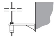
Angular bracket with facade tightener
